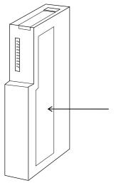
Jumper plugs for selecting the input delay are provided. Refer to section 3.1.
